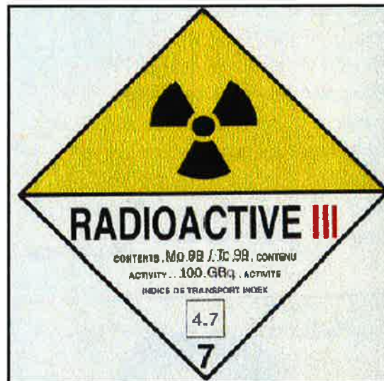
Figure 1: Example of III-Yellow label shows a Transport Index of 4.7
